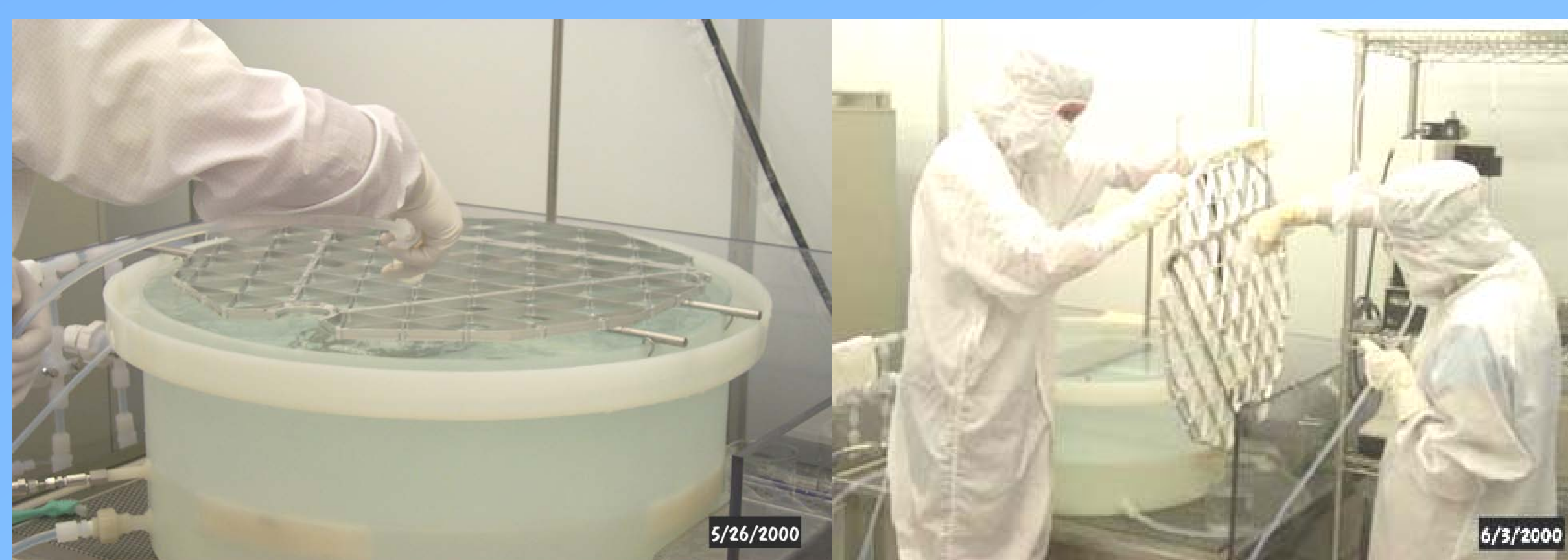
Ultrapure Water and Ultrasonic Cleaning and Inspection of the array collector grids.
