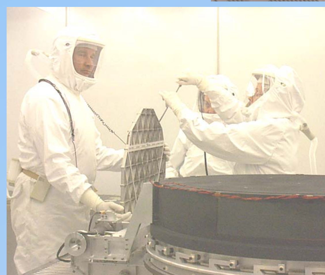
Installation of nine ultrapure hexagonal array materials for solar wind regime capture.
