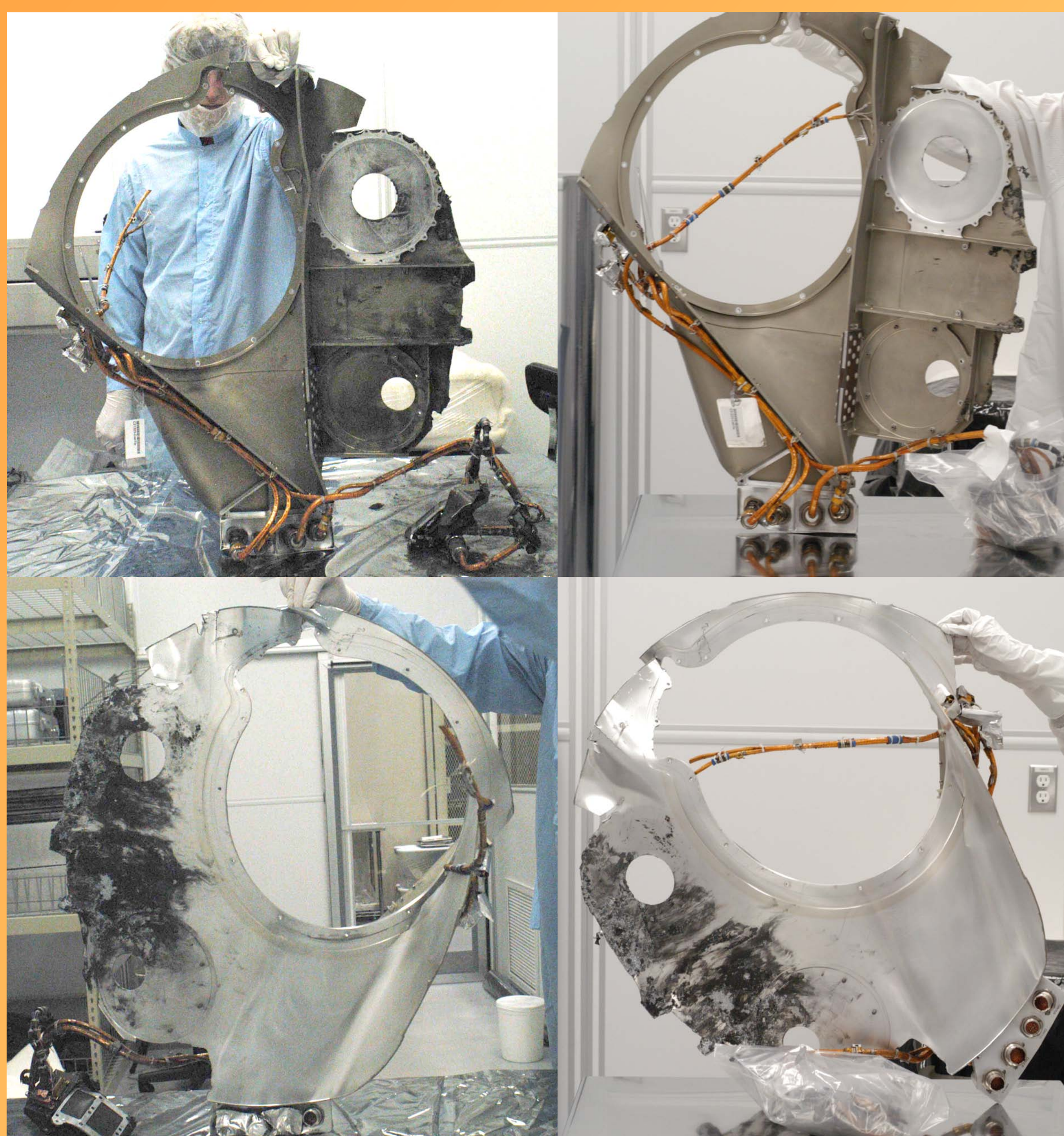
Exterior (above) and interior (below) views of the science canister base before cleaning (left) and after cleaning (right).
