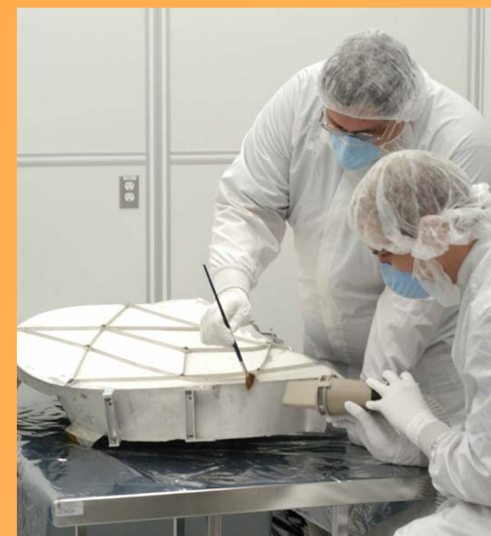
The cleaning process consisted of gentle sweeping and vacuuming of fine particles.
