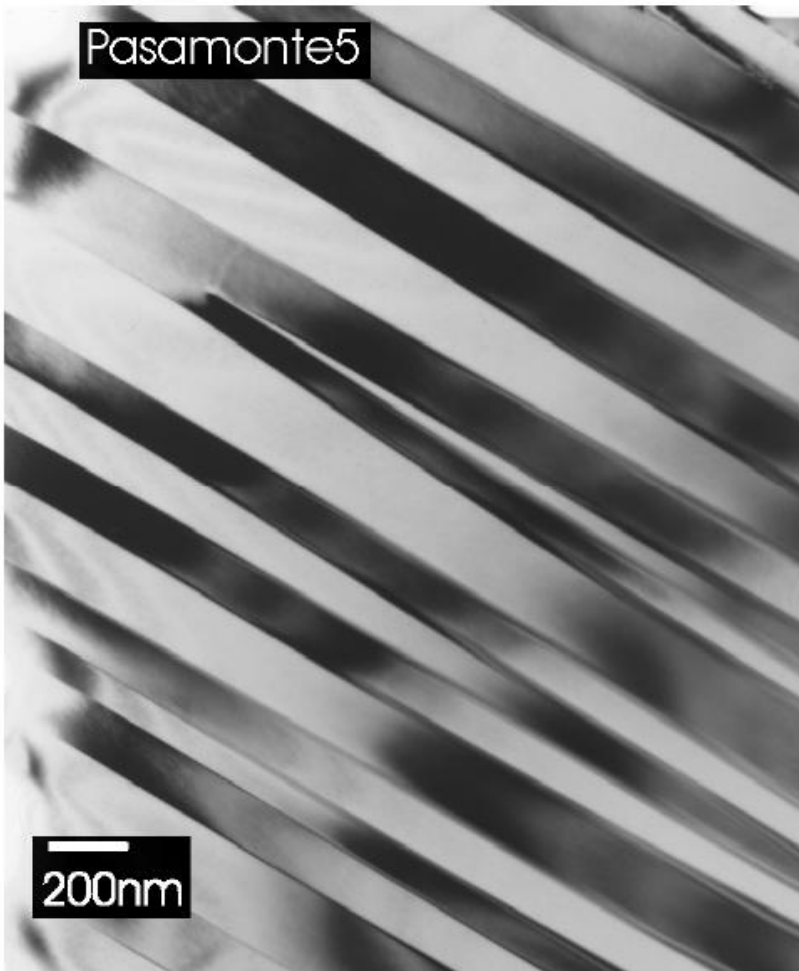
Figure 20: TEM image of (001) augite lamellae (dark) in Pasamonte pigeonite (light); these lamellae have a wavelength of 225 nm. From Schwartz et al (2002).
