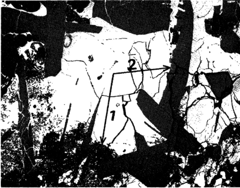
Figure 18: Type 1 and 2 zoning observed in the same pyroxene crystal, from Miyamoto et al (1985); transect 1 ends in a mesostasis and transect 2 terminates in a plagioclase lath.
