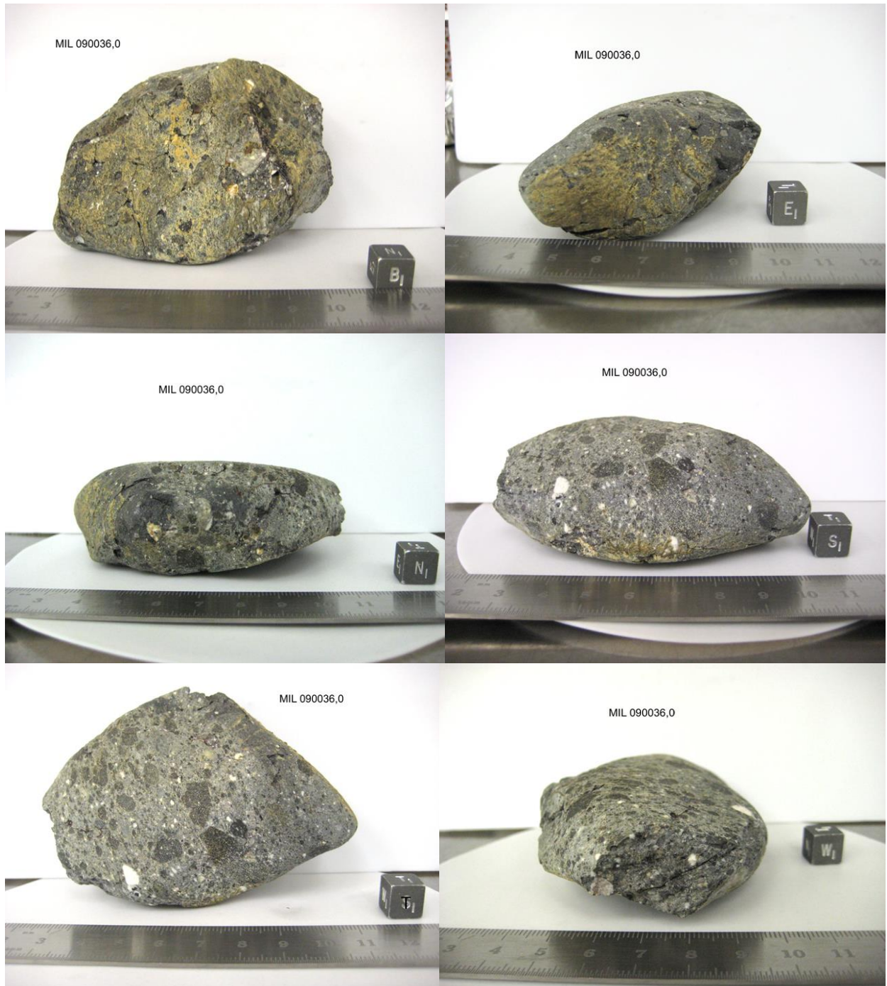
Figure 3: Orthogonal views of lunar meteorite MIL 090036, illustrating the yellowish-brown fusion crust, and brecciated interior including many clearly feldspathic (white) clasts and mineral fragments.
