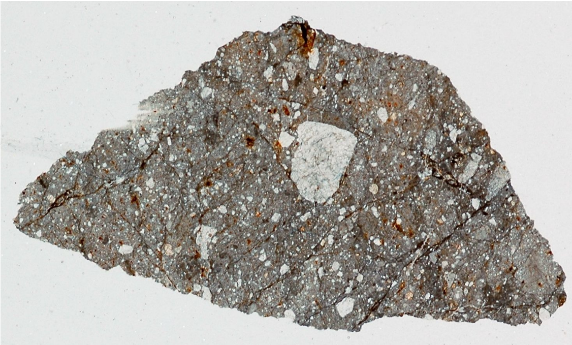
Figure 3: Thin slice through SaU 300 illustrating the overall texture and size and nature of the clasts and fragments (from Hsu et al., 2008 and Bartoschewitz and Korotev, 2010).
