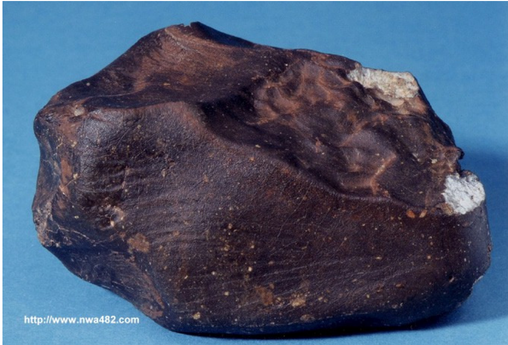
Figure 1: NWA 482 showing brown crust that is both terrestrial weathering (varnish) and fusion crust. Sample is approximately 10 cm in width.
