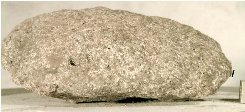
Figure 2: Side view of 77535 showing rounded surface caused by long term micrometeorite bombardment. Cube is 1 cm. S73-19124.
