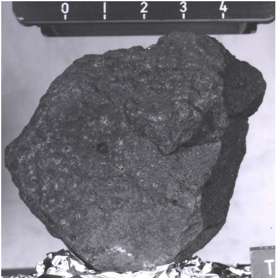
Figure 7: Original photo of 70255 showing large micrometeorite crater. Scale is in cm. NASA S73-24101.
