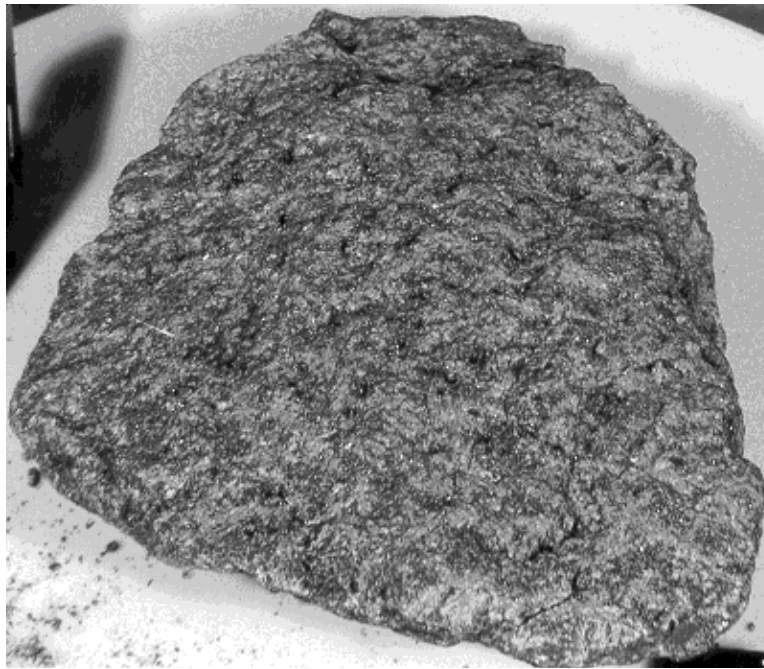
Figure 11: Another view of 15536 showing fresh hackly surface. NASA S71-60585. Sample is 9 cm.
