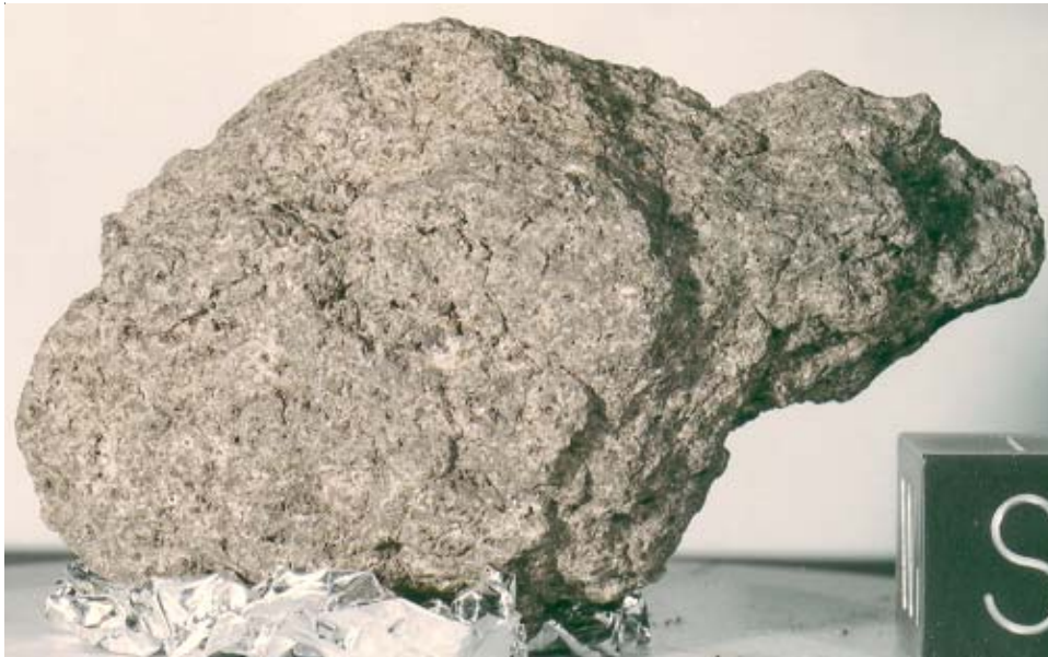
Figure 1: Exterior surface of 15535 (known as the Bear). NASA S71-47029. Cube is 1 inch for scale. Note zap pits.
