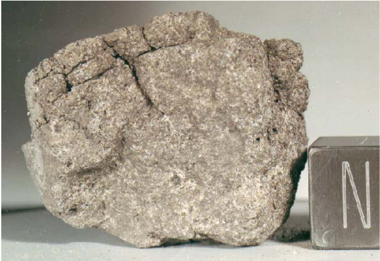
Figure 1: PET photo of top surface of 14053 showing micrometeorite craters. Cube is 1 inch high. NASA photo # S71-35849.
