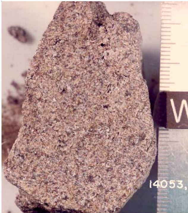
Figure 3: Freshly sawn interior surface of 14053 showing basaltic texture. Cube is 1 cm. Photo # S75-33971.
