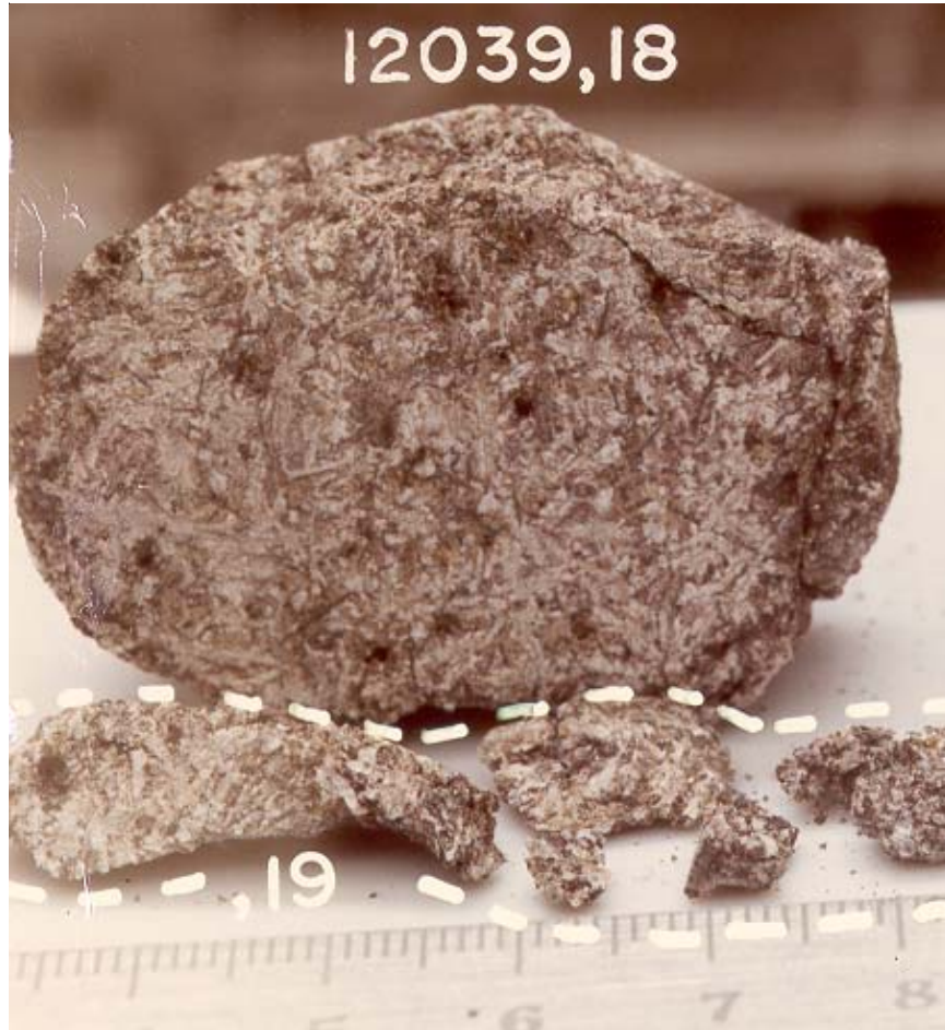
Figure 1: Photo of sawn surface of 12039,18 showing coarse-grained, basaltic textures. Ruler is marked in cm. NASA #S75-34141.
