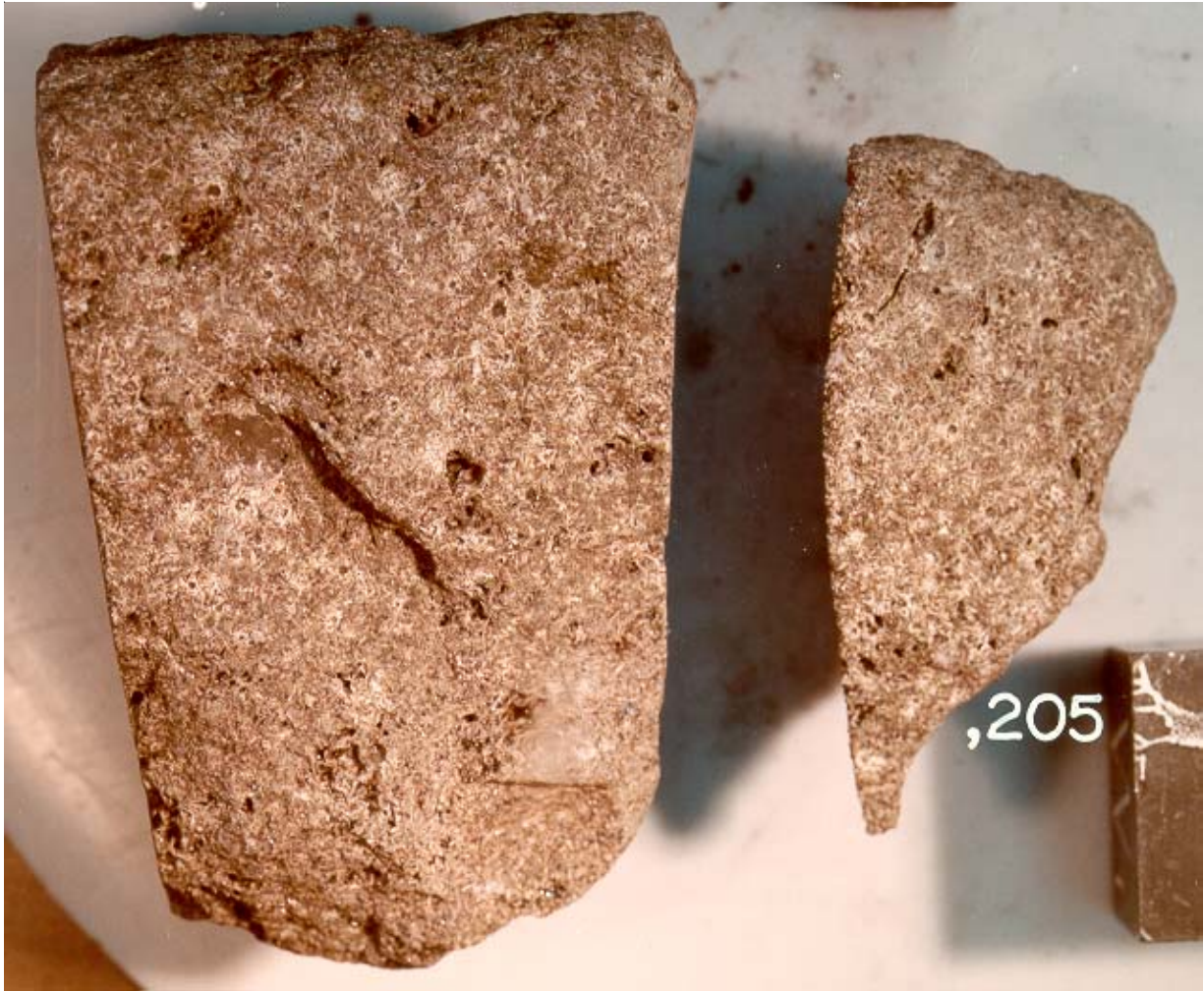
Figure 1: Picture of surface of 12038,7 and ,205 showing zap pits. Cube is 1 inch. NASA #S75-34403.
