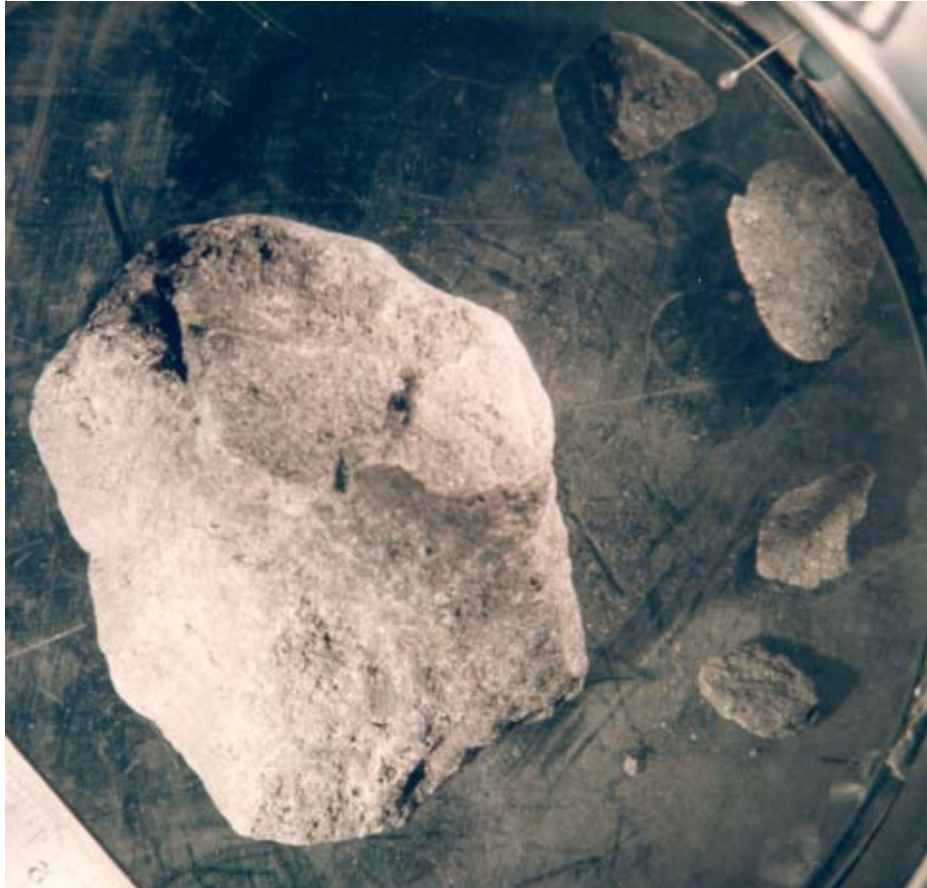
Figure 1: Original “mug shot” for 12018 PET showing main pieces and smaller pieces. NASA #S69-64111. Note the apparent encrustation.
