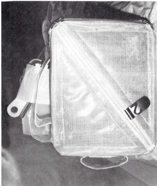
Fig. 98. Top of closed Sample Collection Bag The fabric texture and the diagonal slit through which samples could be dropped is visible. The white fabric in the background is part of the seal protector for the ALSRC (NASA photo S88-52673).
