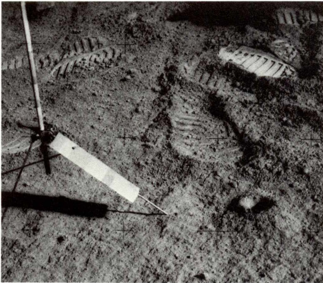
Fig. 14. Hole remaining in lunar regolith after drive tube in previous photo was removed (NASA photo AS15-82-11163).
