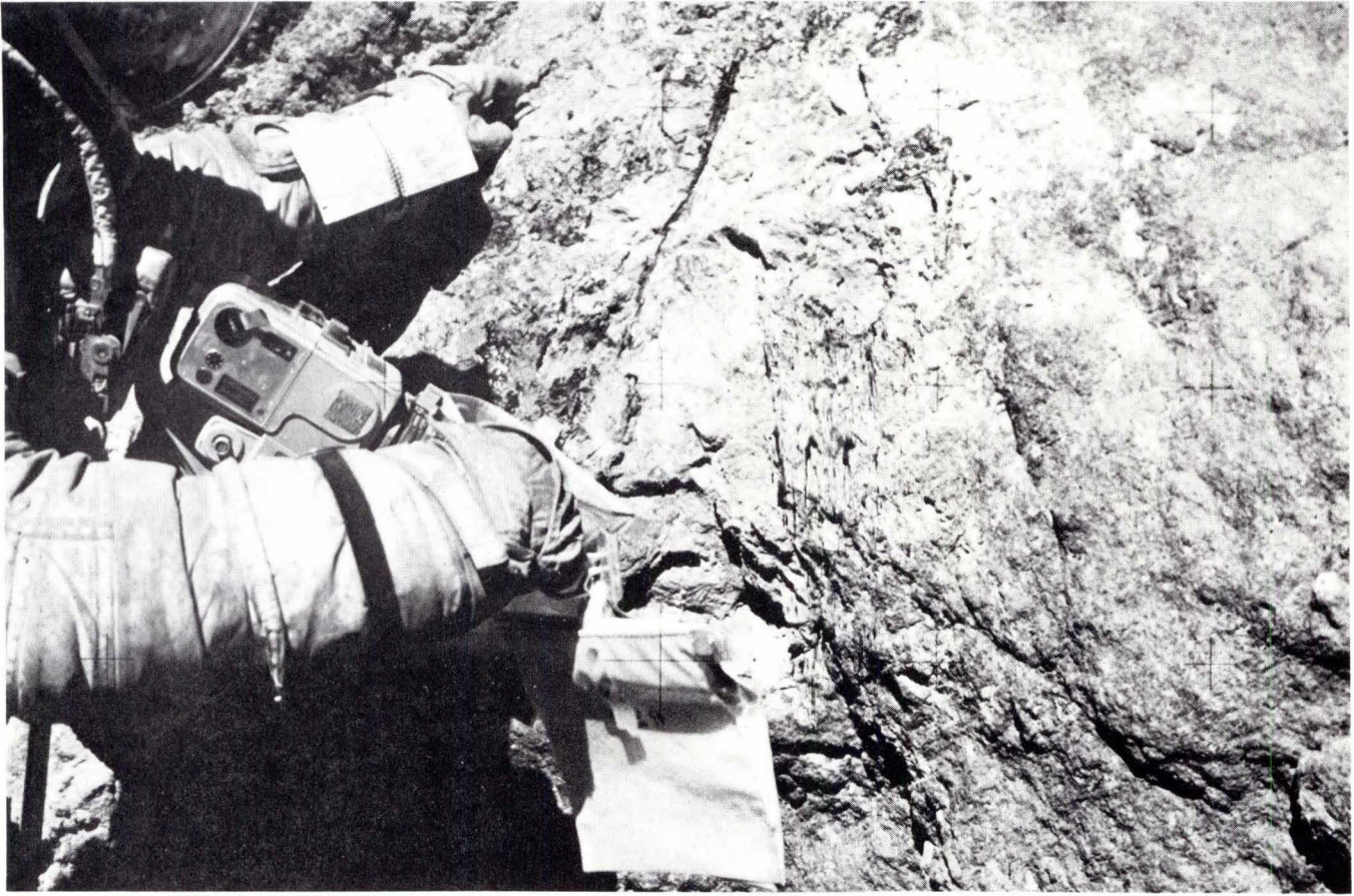
Fig. 85. Apollo 16 astronaut examines large boulder with a 20-bag dispenser attached to his right wrist (NASA photo AS16-116-18649).
