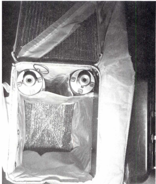
Fig. 99. View into open Sample Collection Bag . Two drive tubes are placed in the interior pockets. The metal mesh stiffener in the lid and in the bottom and the underside of the diagonal slit are visible in the lid (NASA photo S88-52671).
