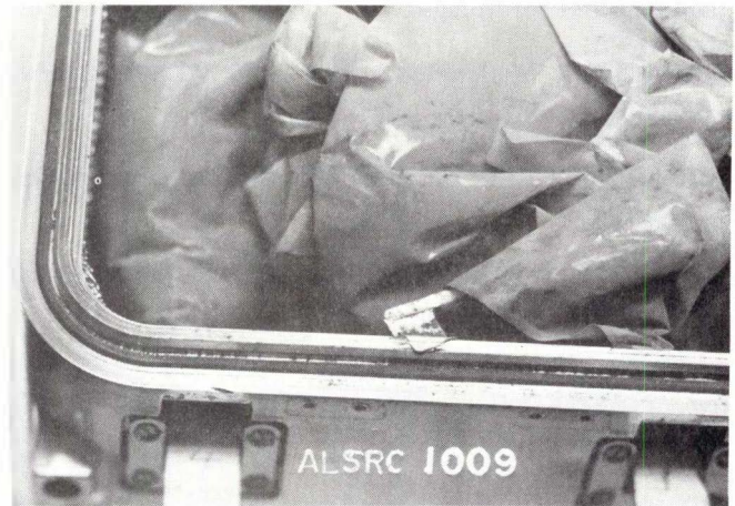
Fig. 75. Close-up view of indium seal in rock box full of lunar samples in documented sample bags. The aluminum tab on one of the bags was entrapped in the knife-edge and indium seal; thus, the seal was not good. One of the fluorosilicone o-rings, dark in color, is visible just outward of the indium seal (NASA photo S72-37750).
