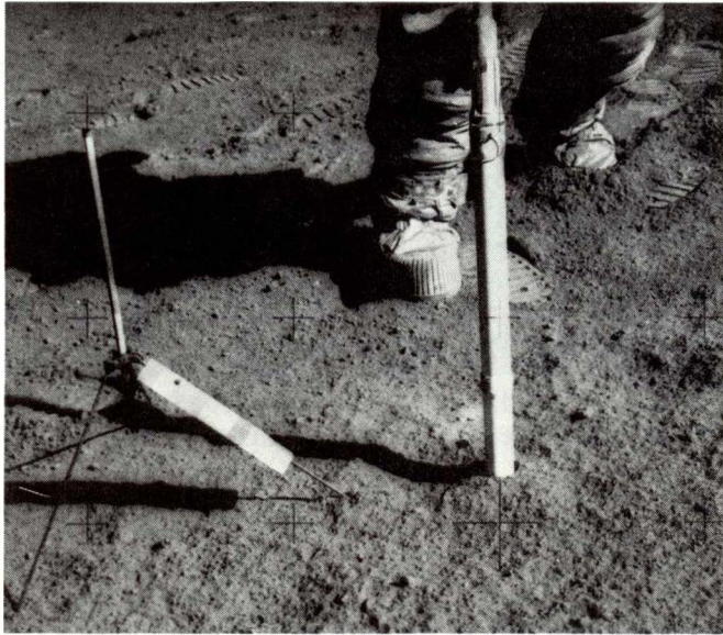
Fig. 13. A double length drive tube attached to an extension handle is being driven by an Apollo 15 astronaut. The top one-third of a lower tube, an entire upper tube, and the bottom portion of an extension handle are visible (NASA photo AS15-82-11161).
