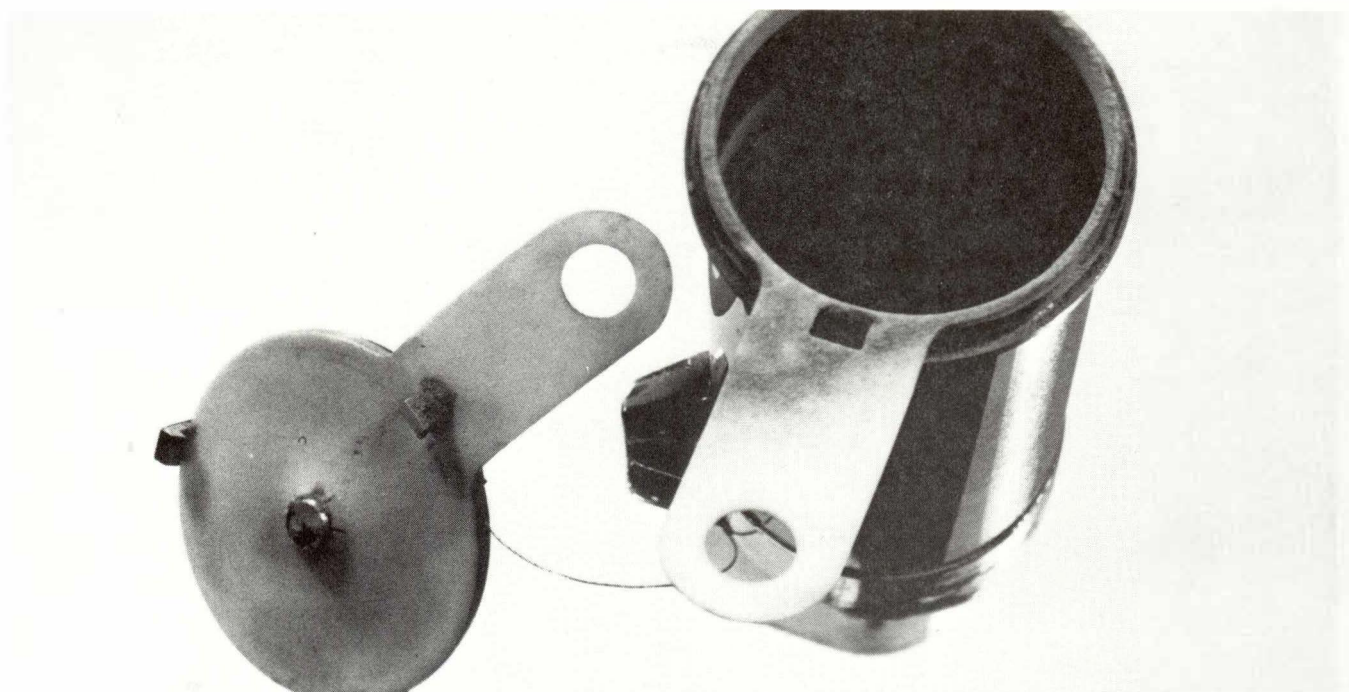
Fig. 93. SESC, with seal protectors in place, after being filled with simulated lunar dust in an experiment to test the ability of the seal protectors to keep the sealing surfaces clean (NASA photo S88-52667, taken from Union Carbide photo no. 137775).
