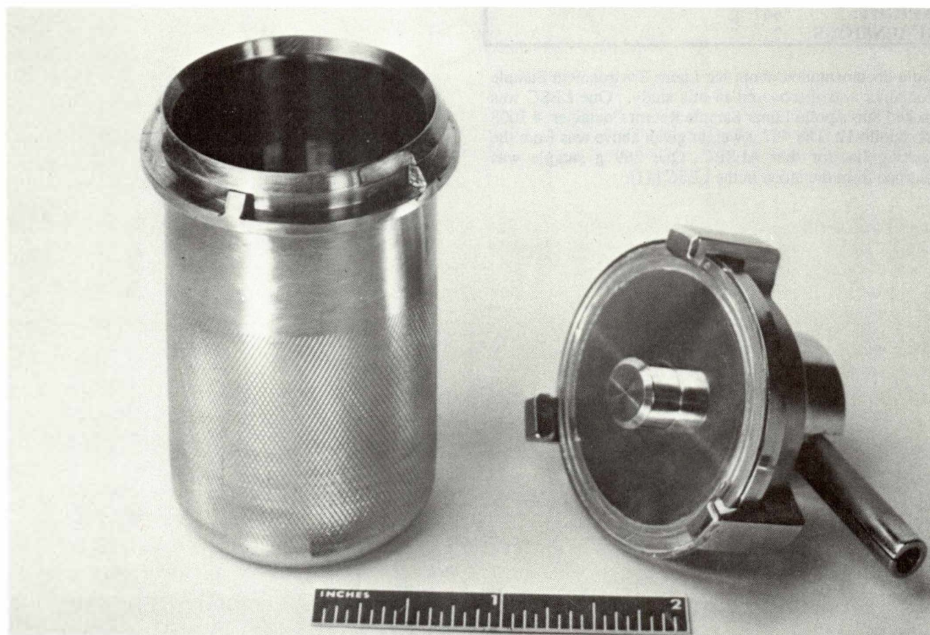
Fig. 86. Gas Analysis Sample Container (GASC). The knife-edge on the can and indium alloy sealing surface on the lid are visible (NASA photo S88-52660 taken from Union Carbide photo no. 121372).
