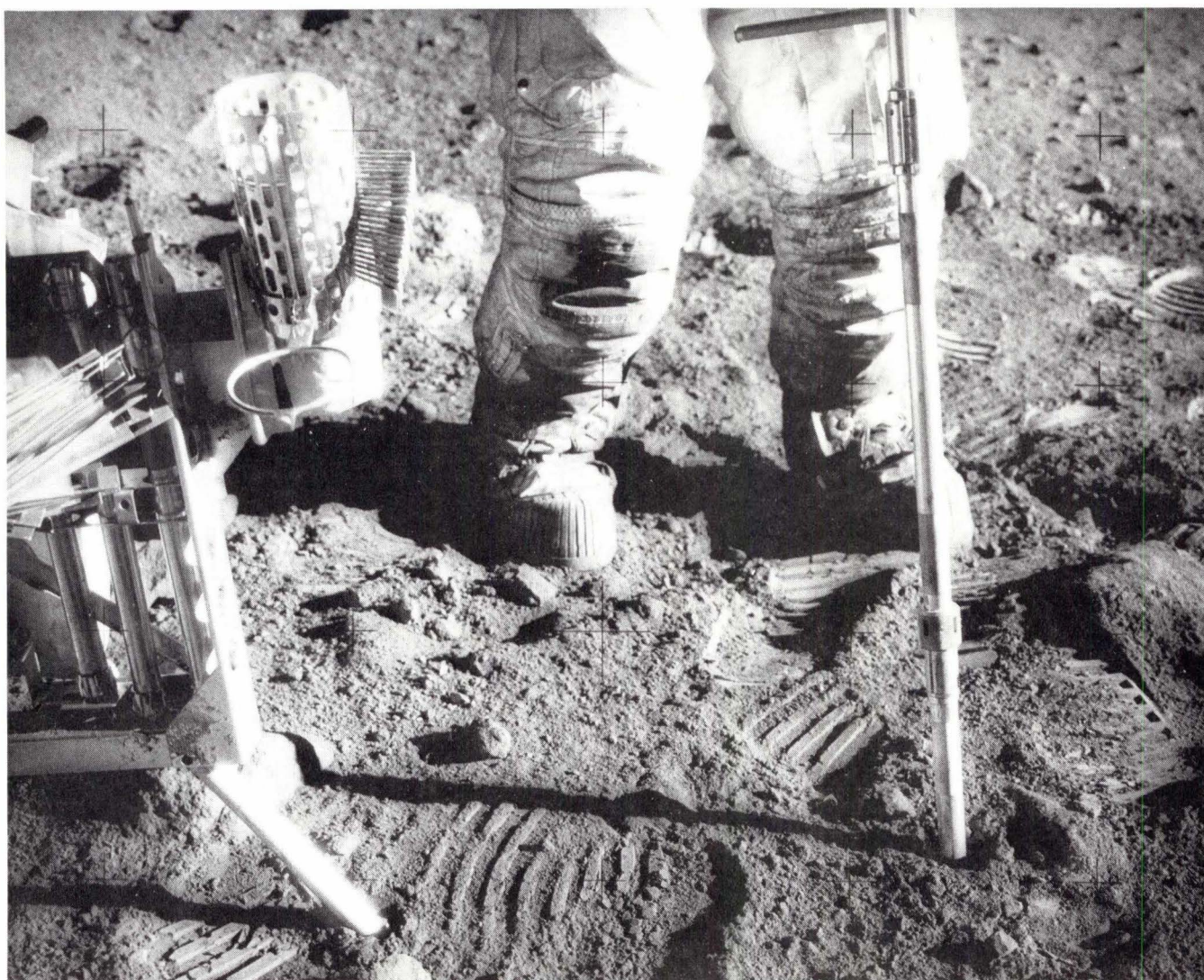
Fig. 77. Cup-shaped documented sample bags in 35-bag dispenser hanging on small tool carrier at Apollo 12 site (NASA photo AS12-49-7243).
