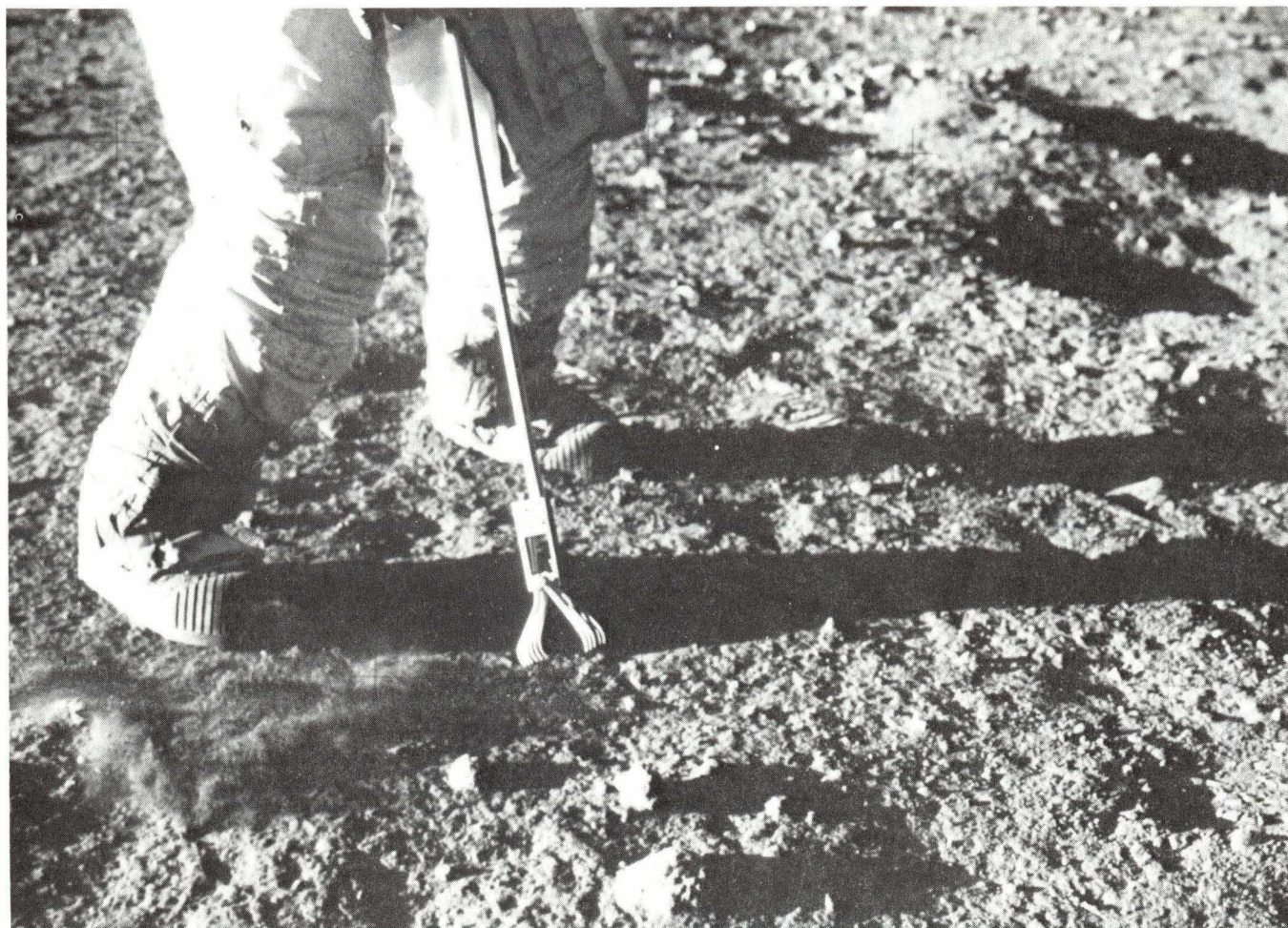
Fig. 48. Shorter model tongs in use during Apollo 12 mission (NASA photo AS12-47-6932).
