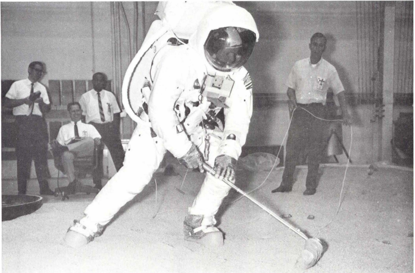
Fig. 5. Space-suited person testing contingency soil sampler in simulated lunar regolith (NASA photo S69-31048).
