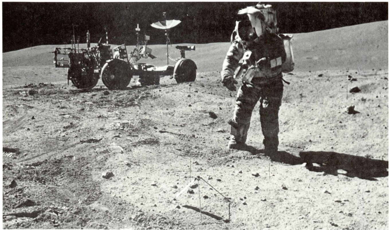
Fig 68. Apollo 16 lunar rover with large tool carrier opened outward to allow access to tools on both sides of the carrier (NASA photo AS16-117-18825).
