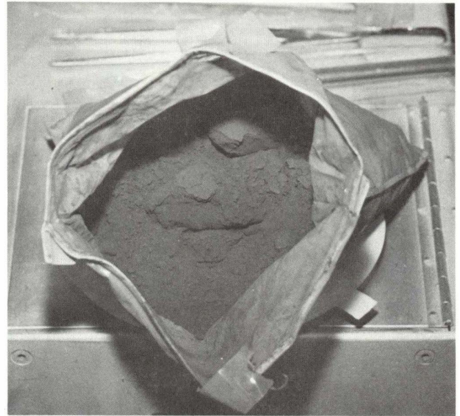
Fig. 83. Flat, rectangular documented sample bag opened in laboratory to show Apollo 17 soil 74220, weighing 1180 g. The aluminum rim holds the bag open (NASA photo S73-15561). 573-15061
