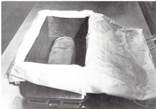
Fig. 74. Teflon cloth seal protector, deployed as if on lunar surface, during packing of ALSRC prior to flight. The box lining is York mesh (NASA photo S88-52674).
