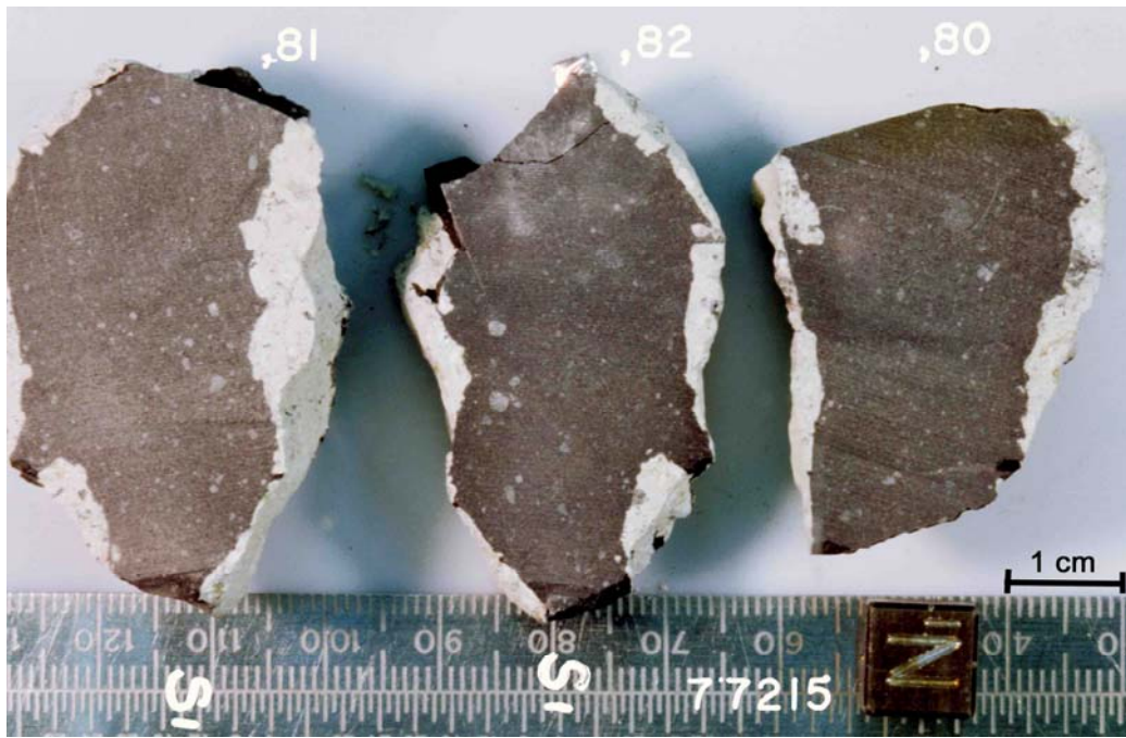
Figure 2: Photograph of sawn surfaces of slab and butt ends of 77215,19. Cube is 1 cm. S75-21992.
