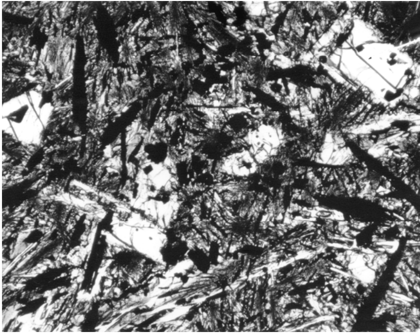
Figure 2: Photomicrograph of 71589,4. Olivine and ilmenite phenocrysts set in a sub-variolitic to variolitic ground mass. Field of view = 2.5 mm.
