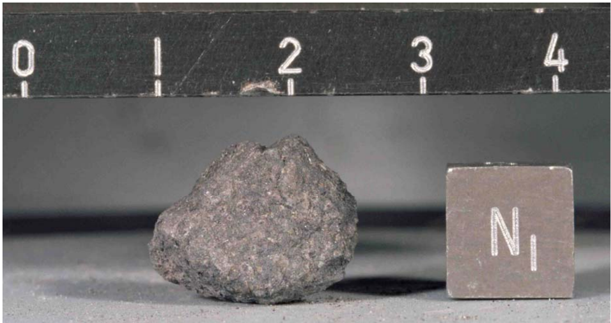
Figure 1: 73219, pre-processing. Cube and scale divisions are 1 centimeter. S-73-16963.
