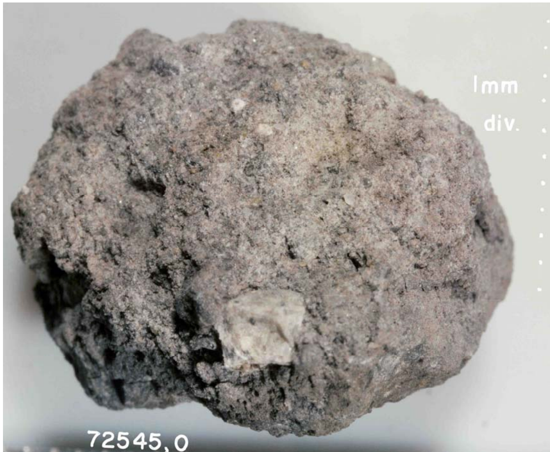
Figure 1: Sample 72545, showing prominent plagioclase or feldspathic fragment. Small scale divisions in millimeters. S-73-19625.
