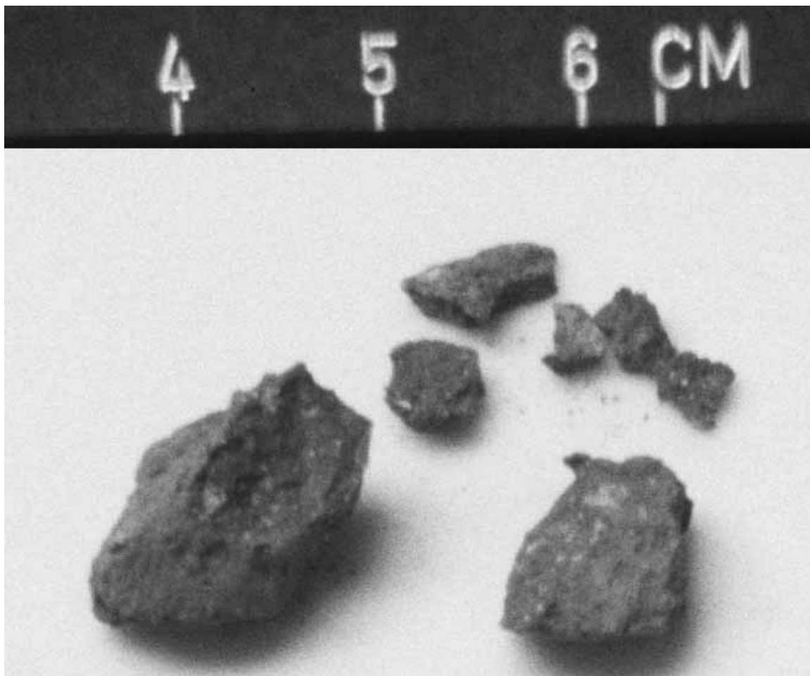
Figure 1. Post-chip view of 15326. Largest piece is ,0; second largest is ,1, used for thin sections. S-71-57228
