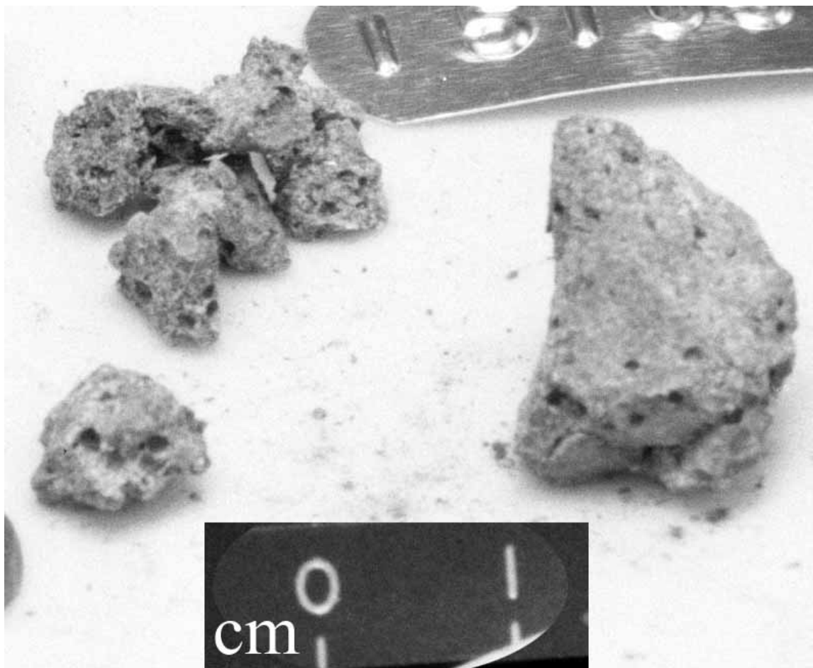
Figure 1. Post-chipping view of 15105. The front chip ,2 was potted and thin section ,6 made from it. S-72-20376
